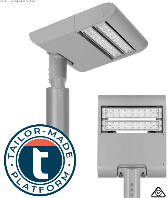
Top right and below: 64 Tiger Streetlights deployed in the vicinity of the regional airport, requiring minimal upward and lateral light spill, due to CASA regulations. Warm white lighting was specified with a CRI above 80. The luminaires ranged in output from 40W to 120W, with DALI control to allow operation to be scheduled and output to be dimmed as required.
