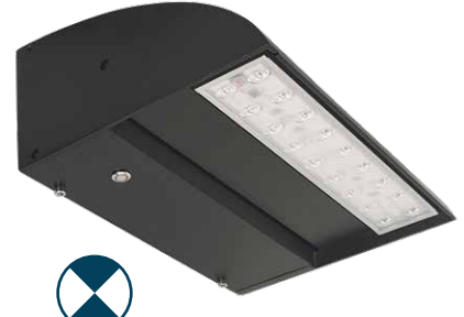
SENTRY EMERGENCY 40W 6000lm / 589 lm. Maintained emergency External self test button Run-time 3hrs @ 5W Weight 3.7kg. WLC040L-EM
