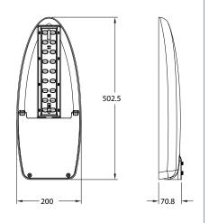
SIZE: 495mm L x 200mm W x 75mm H WEIGHT: 5.88kg EPA: 0.076m2
