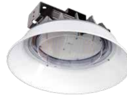
Optional 115 degree reflector reduces glare at low ceiling heights. 50 deg also available.
